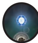
Blue LED indicates valve is receiving control voltage and should be in the open position.
