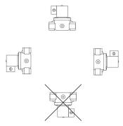
Metal shoe construction of the diaphragm allows for vertical installation, with less damage from debris and over pressure.
