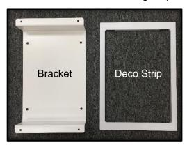
The bracket is designed to cradle the Merlin control panel and hold it securely in place within a standard constructed inner wall. The wings of the bracket should sit on to stud work, leaving the fascia panel proud of the finished surface. The Decorative strip is intended to cover up any cut-in work and any hardware used to fix the bracket in place.
