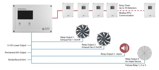
Addressable AGS TFT detectors are daisy-chained through a RS-485 RTU communication protocol to the controller. The controller must be installed and located in accordance with applicable regulations, out of reach of the public, close to the motor control centre or in connecting offices.
