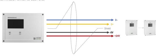
Recommended 3-core, 2 twisted pair + ground, shielded cable with 120  $\Omega$  characteristic impedance.
