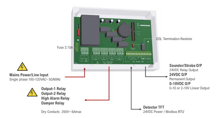
**Power/Line Input** The controller requires a single-phase power supply of 100-120VAC. When power is introduced to the controller, a red LED will illuminate on the front of the controller (AGS Logo) and the screen will power up.
