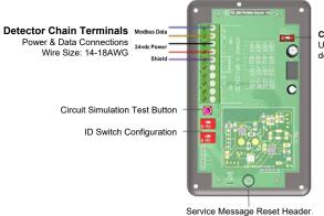
Chain Termination Resistor Used to select the first and last device in the chain
