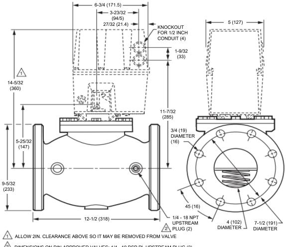
DIMENSIONS ON DIN-APPROVED VALVES: 1/4 - 19 BSP.PL UPSTREAM PLUG (2), .71 IN DIAMETER BOLT HOLE (16), 7.087 IN DIAMETER BOLT CIRCLE.
