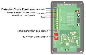
Chain Termination Resistor Used to select the first and last device in the chain
