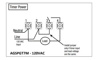
Tungsten: 5 Amps @ 120/240 VAC Ballast: 20 Amps @ 120-277 VAC
