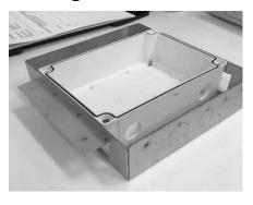
Fold out wing brackets for framed installation. The wings provide a ½" space to allow for drywall install.
