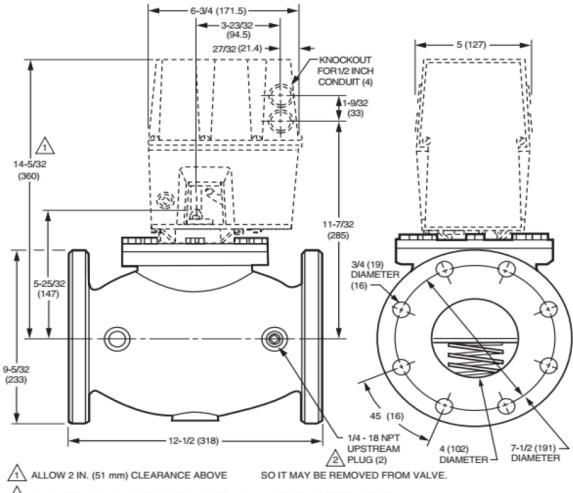
DIMENSIONS ON DIN-APPROVED VALVES: 1/4 - 19 BSP.PL UPSTREAM PLUG (2), .71 IN (18 mm) DIAMETER BOLT HOLE (16), 7.087 IN (180 mm) DIAMETER BOLT CIRCLE.
