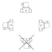
Metal shoe construction of the diaphragm allows for vertical installation, with less damage from debris and over pressure.
