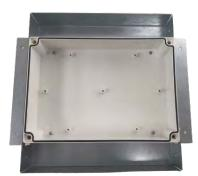
Fold out wing brackets for framed installation. The wings provide a  $\frac{1}{2}$ " space to allow for drywall install.
