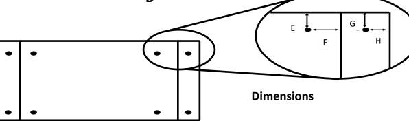
The wings of the bracket are designed to be mounted on to the drywall of the finished surface. If the finished surface is other than drywall the depth of installation should be calculated to compensate for the finished surface.
