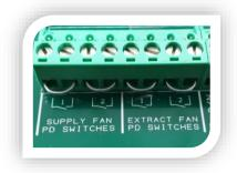
Wiring to switches & current monitors should be made using two-core volt free connections.
