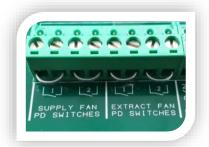
Wiring to switches & current monitors should be made using two-core volt free connections.
