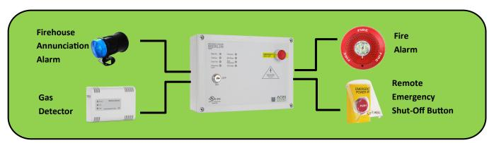
An "off" delay function can be added to the system with the addition of the AGSFAB1 bypass panel, allowing personal to activate a bypass of the shut-down within 60 seconds of the annunciation alarm sounding. If the bypass is not activated within the initial 60 seconds the Merlin unit will de-energize the gas supply. Additional safeguards include the AGS gas detectors and built-in time options.
