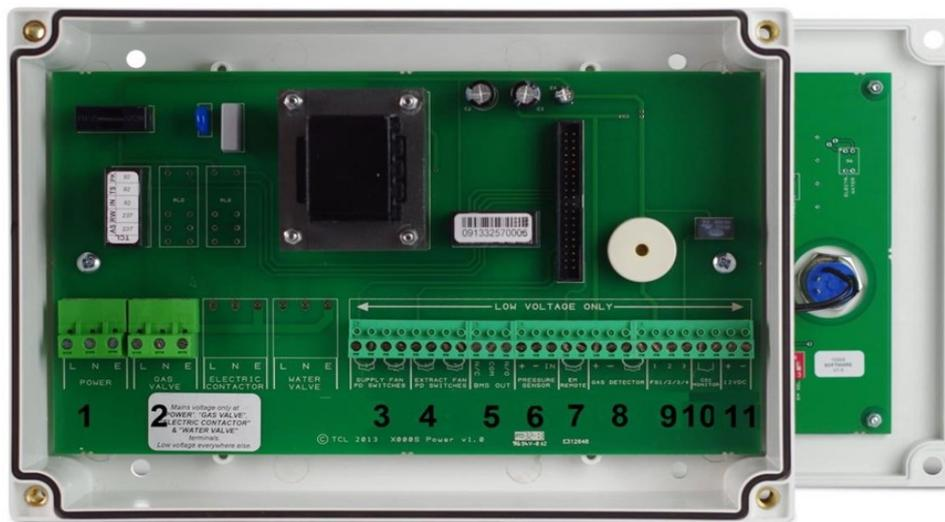
1. Mains Supply Input, Single phase 100/240VAC 50/60HZ
