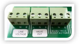
An electrical output can be supplied to an electrical contractor. This should be fused at 3A and connected to the terminals marked [ELECTRIC CONTACTOR LNE].
